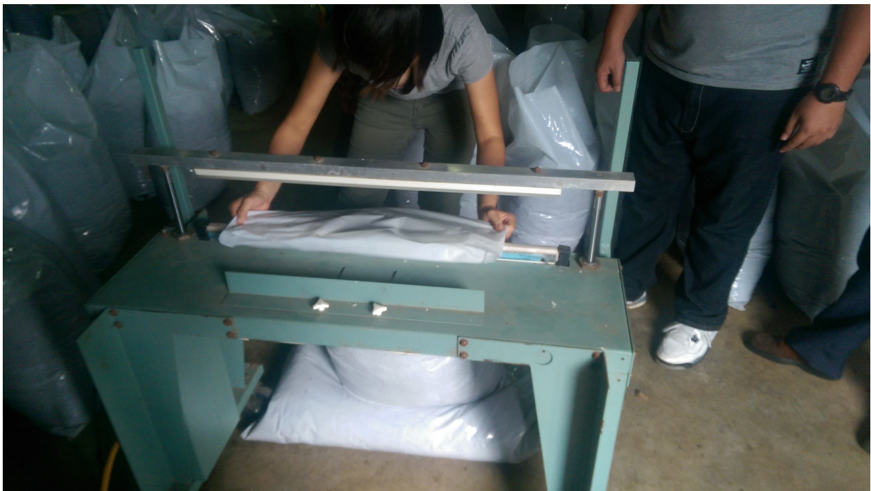
Image 4. Hot sealing NWP-assigned bulk bags
